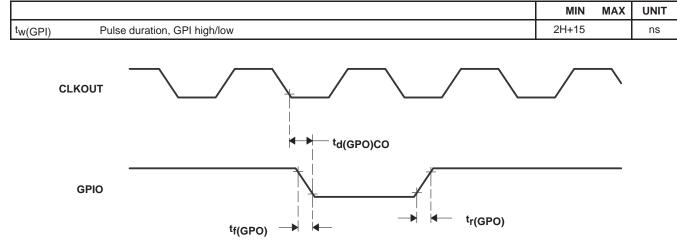
Figure 37. General-Purpose Output Timing
