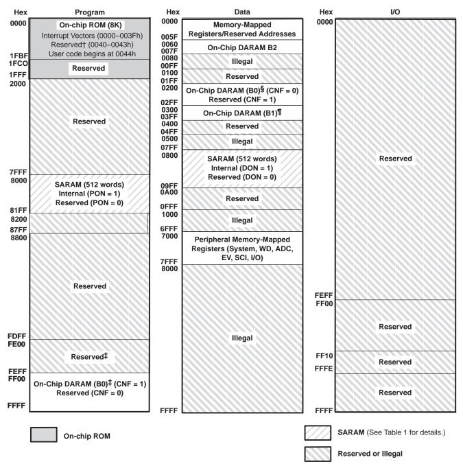
NOTE A: Boot ROM: If the boot ROM is enabled, then addresses 0000–00FF in the program space will be occupied by boot ROM. <sup>†</sup> Addresses 0040h–0043h in program memory are reserved for code security passwords.
