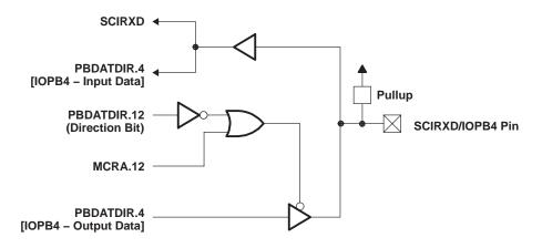
Figure 6. SCIRXD/IOPB4 Pin Multiplexing Functional Block Diagram
