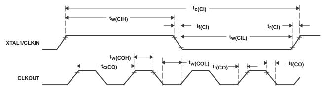
Figure 26. CLKIN-to-CLKOUT Timing With PLL and External Clock in ×4 Mode
