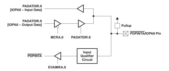
Figure 2. PDPINTA/IOPA0 Pin Multiplexing Functional Block Diagram
