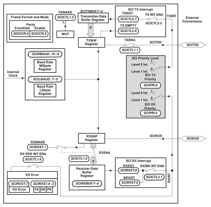
Figure 16. Serial Communications Interface (SCI) Module Block Diagram
