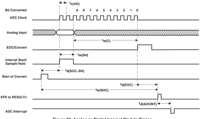
Figure 39. Analog-to-Digital Internal Module Timing
