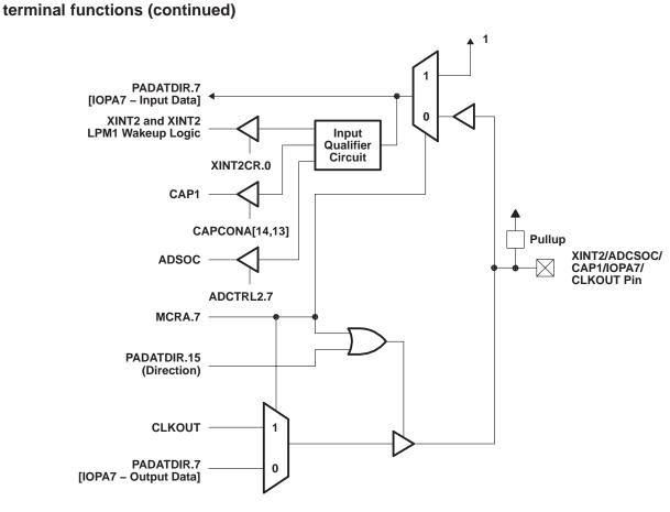
Figure 3. XINT2/ADCSOC/CAP1/IOPA7/CLKOUT Pin Multiplexing Functional Block Diagram
