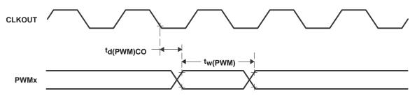
Figure 34. PWM Output Timing
