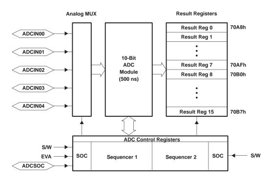
Figure 15. Block Diagram of the 2401A ADC Module
