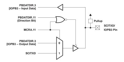
Figure 5. SCITXD/IOPB3 Pin Multiplexing Functional Block Diagram
