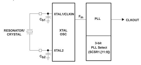
Figure 17. PLL Clock Module Block Diagram
